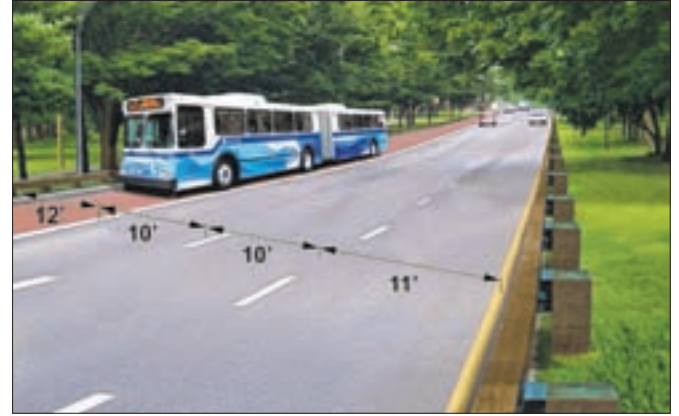
A rendering of the proposed changes to the Pelham Parkway Westbound Mainline, as part of phase two of the reconstruction of Pelham Parkway. A dedicated bus lane will be added by shifting the existing lanes and eliminating the shoulders.
