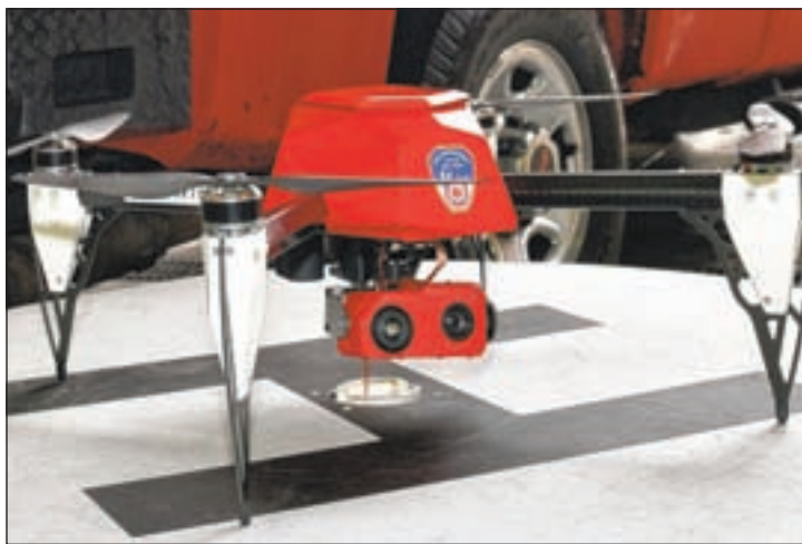
The FDNY used this state-of-the-art tethered drone equipped with high definition and infrared cameras to determine the condition of Crotona Park North's roof as they contained the blaze.
