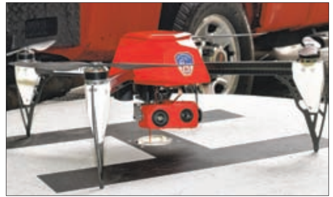
The FDNY used this state-of-the-art tethered drone equipped with high definition and infrared cameras to determine the condition of Crotona Park North's roof as they contained the blaze.
